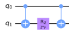
Figure 2.21: Cost layer- apply 2 CNOT gates and an R_z gate (decomposition of R_{zz} gate)
